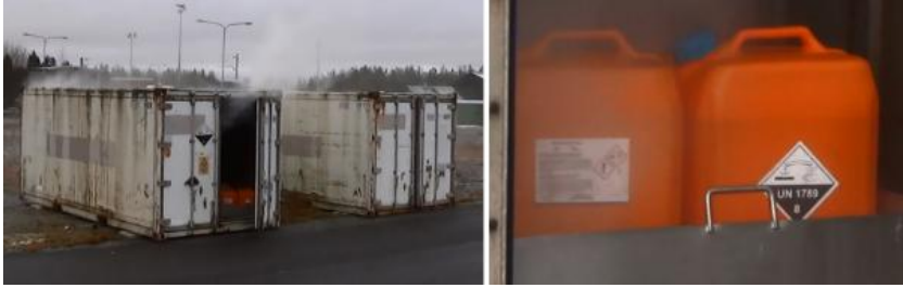
Figure 114. Extractions from the AIF video of Videodrone X8 drone during the identification of acid containers inside the container. UN 1789 8 stands for hydrochloric acid (HCl).
