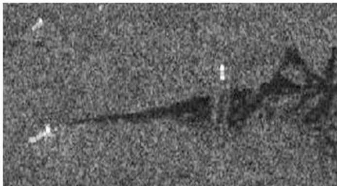
Figure 18. SAR image of a ship (bright target near the bottom left corner) discharging oil into the sea. (Centre for Remote Imaging, Sensing and Processing (CRISP), 2015)
