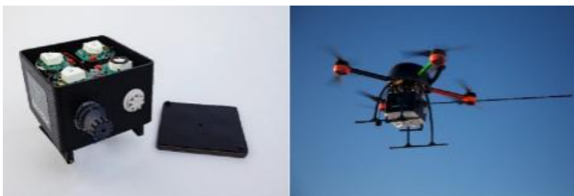
Figure 95. Aeromon BH-8 module with its lid open (left) and mounted on a drone (right). (Aeromon, 2016)
