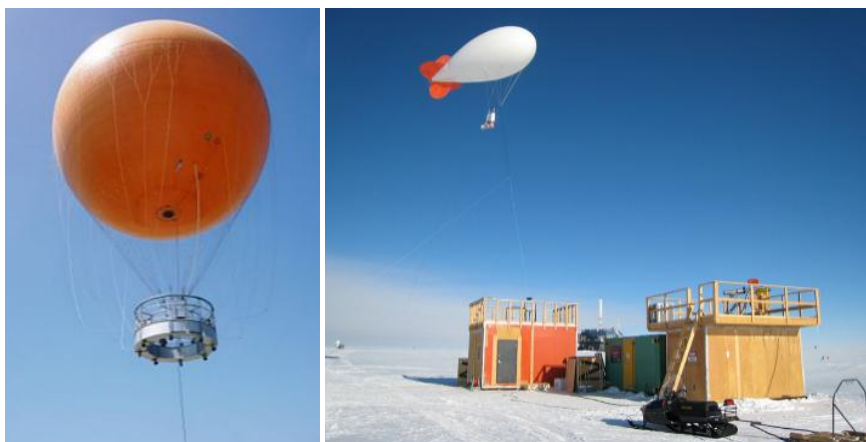
Figure 46. Examples of tethered balloon systems: Aerophile Group (left), and SPEC Ltd ready for deployment at the South Pole (right).
