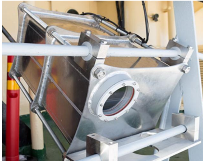
Figure 67. Light Detection and Ranging (LiDAR) oil spill detection system by Ocean Visuals AS during the Kemi Arctic 2015 exercise. (Image: SYKE/Jyrki Nikkilä)
