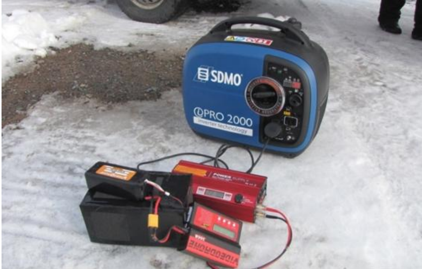
Figure 61. The inverter charging the batteries of the UAS. (Image: VTT/Jukka Sassi)
