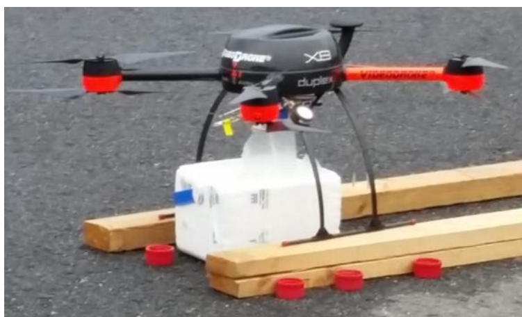
Figure 110. The drone with the sorbent tube, sampling pump and 3M passive sampler after landing over the polystyrene box for sampling. (Image: VTT/Jukka Sassi)
