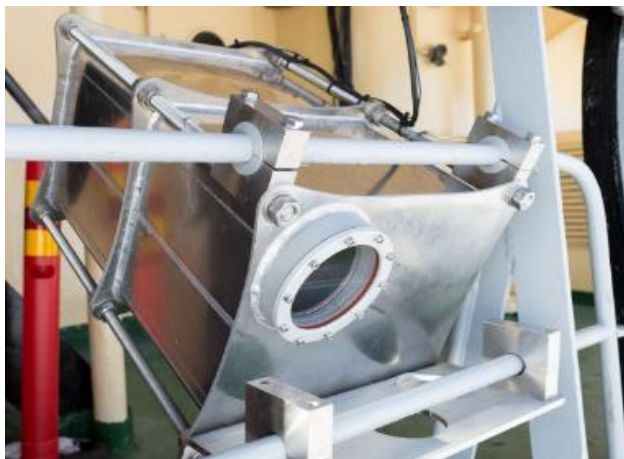
Figure 23. Light Detection and Ranging (LiDAR) oil spill detection system by Ocean Visuals AS. (Image: SYKE/Jyrki Nikkilä)
