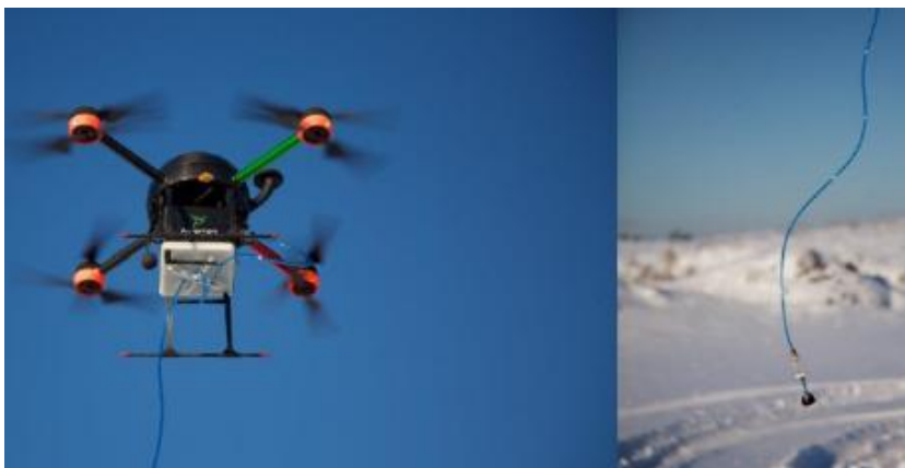
Figure 99. 10 m long polyurethane tube with a filter unit (right) attached to the sample intake. (Images: Aeromon, 2016)
