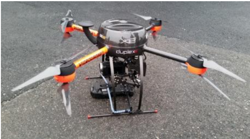
Figure 108. Videodrone X8 with ChemPro100i mounted. (Image: VTT/Jukka Sassi)
