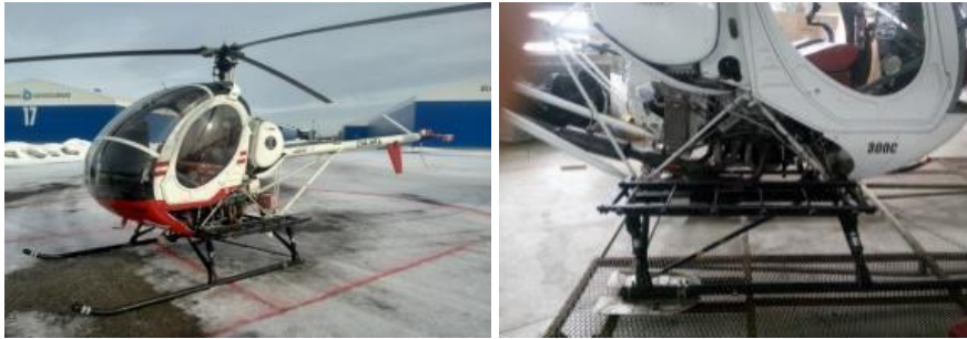
Figure 62. The helicopter ready for test flights. The mounting racks were installed on both sides of the helicopter. (Images: Carelia Copters)
